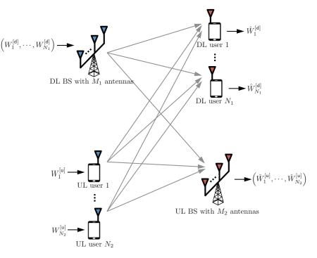
Fig. 6. Two-cell multiantenna cellular networks in which the first and second cells operate as DL and UL respectively.
