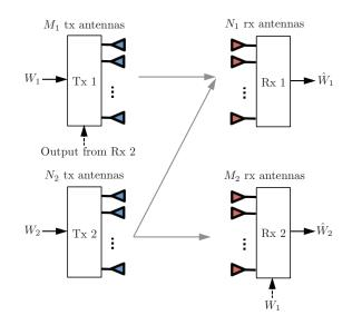
Fig. 9. Two-user MIMO Z-IC with output feedback for encoding and message side information for decoding.
