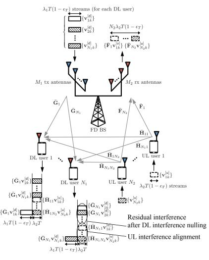
Fig. 7. Conceptual illustration of transmit beamforming for the  $(M_1, M_2, N_1, N_2)$  FD-BS-HD-user cellular network, where for convenience we assume  $\lambda_1 \ge \lambda_2$  in the figure.
