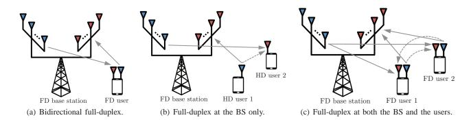
Fig. 1. Full-duplex network configurations.
