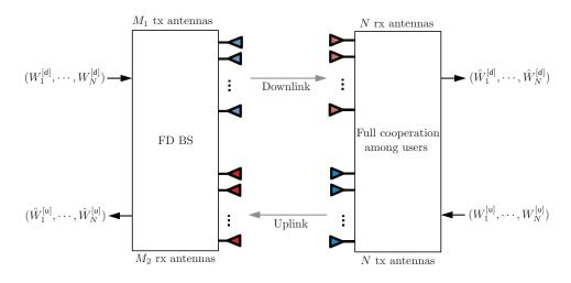
Fig. 10. MIMO two-way channel by allowing full cooperation among the N users.
