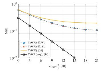
Fig. 6: MU-MISO Downlink 16-QAM MSE using Alg. 1 with  $N_t = 128$  and K = 4, averaged over 200 i.i.d. channels.
