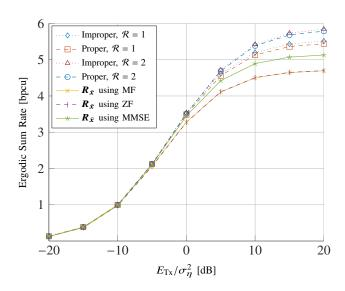
Fig. 3: MU-MISO Downlink lower-bound of the ergodic sum rate with  $N_t = 16$  and K = 2, averaged over 200 i.i.d. channels.
