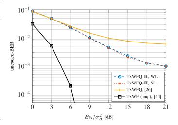
Fig. 5: MU-MISO Downlink 16-QAM uncoded-BER using Alg. 1 with  $N_t = 128$  and K = 4, averaged over 200 i.i.d. channels.
