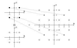
Fig. 4: Linear Superposition Matrix – Two QPSK symbols to one 16–QAM symbol
