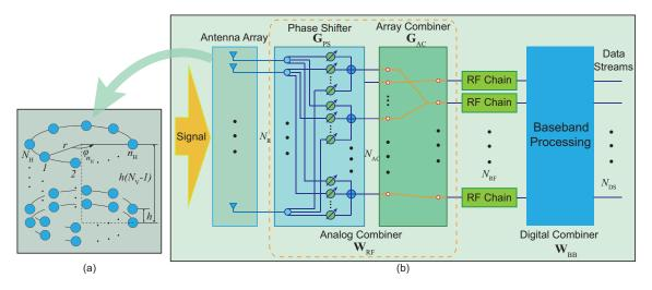
Fig. 2. (a) The geometric model of the UCyA; (b) The block diagram of hybrid beamforming architecture.
