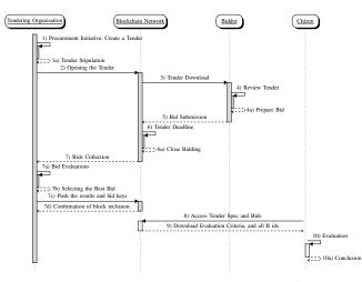
Fig. 3: Smart Contract Based Tendering Architecture
