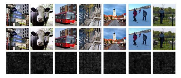
Figure 4: The comparison of the encoded image  $I_e$  (middle row) and the cover image  $I_c$  (top). The bottom row shows the min-max normalized difference between the cover image  $I_c$  and the encoded image  $I_e$ . Additional samples may be found at https://drive.google.com/drive/folders/1sqgAvXcanieYobqzFgt0tkLaVN20pII8
