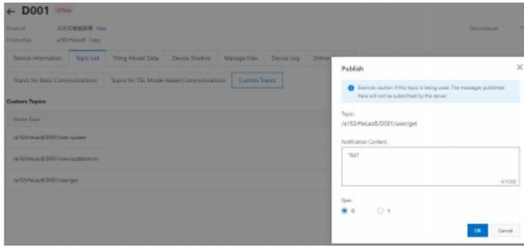
Figure 7 shows the TOPIC list. In the Internet of Things platform, messages are communicated between the server and the device through Topic. Topic is for the concept of equipment, and Topic is for the concept of products. The Topic category of the product will be automatically mapped to all the devices under the product to generate a specific device topic for message communication. The MQTT downlink communication test will use the information release function in the list.
