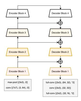
Fig. 1: LinkNet Architecture
