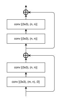
Fig. 2: Convolutional modules in encoder-block (i)
