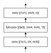
Fig. 3: Convolutional modules in *decoder-block* (i)
