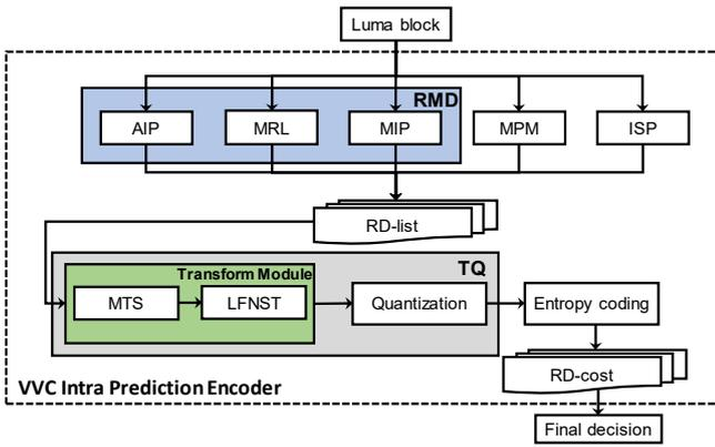
Fig. 1. Encoding flow of the VVC intra-frame prediction for luminance.
