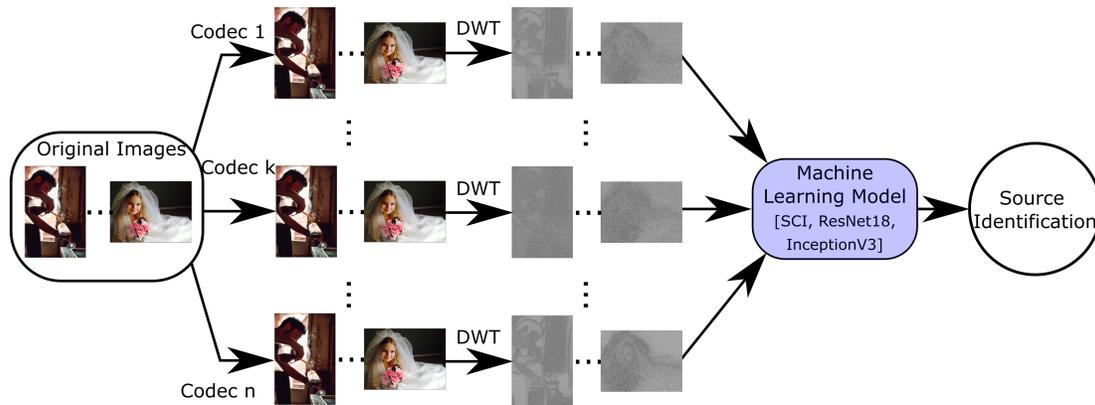
Fig. 2: Overview of the compression source identification pipeline.
