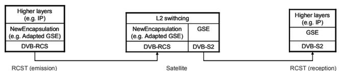
Figure 7: Protocol stacks for on board L2 switching
