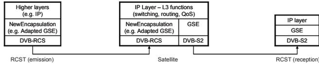
**Figure 8: Protocol stacks for on board L3 switching**
