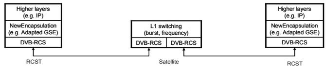
Figure 6: Protocol stacks for on board L1 switching
