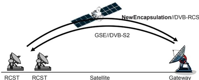
Figure 3: Forward and return link encapsulation
