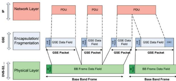
Figure 1: GSE encapsulation by DVB protocol stack [6]
