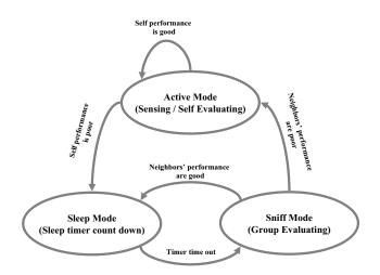
Fig. 1. State diagram of the bio-inspired scheduling scheme.
