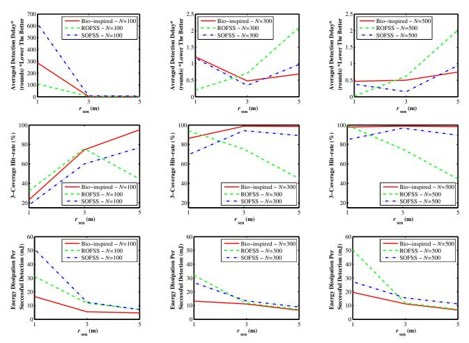
Fig. 2. Performance comparisons of the proposed bio-inspired scheduling scheme, the generic "random on-off" scheduling scheme (ROFSS) and the generic "selective on-off" scheduling scheme (SOFSS) with s = 1 /round,  $r_{\text{eff}} = 3$  m.
