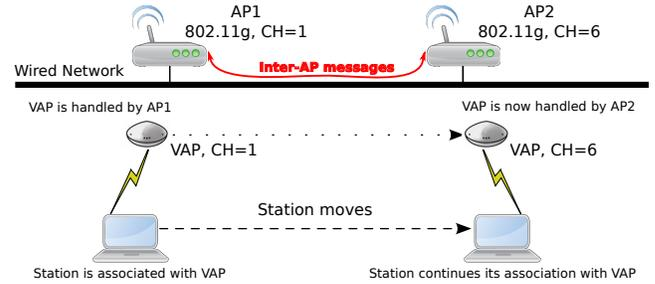
Fig. 1: Mobility management with Multichannel Virtual Access Points
