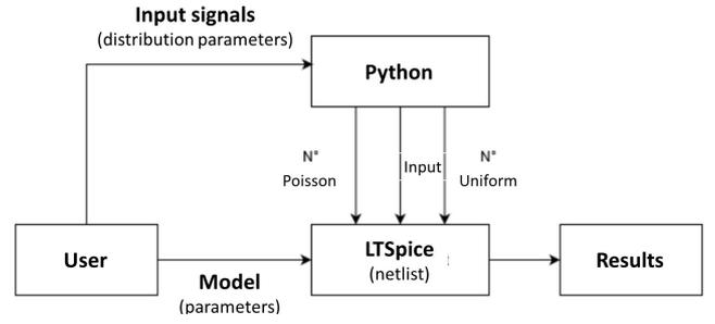
Fig. 2 Block diagram describing the user interaction with the simulation flow.
