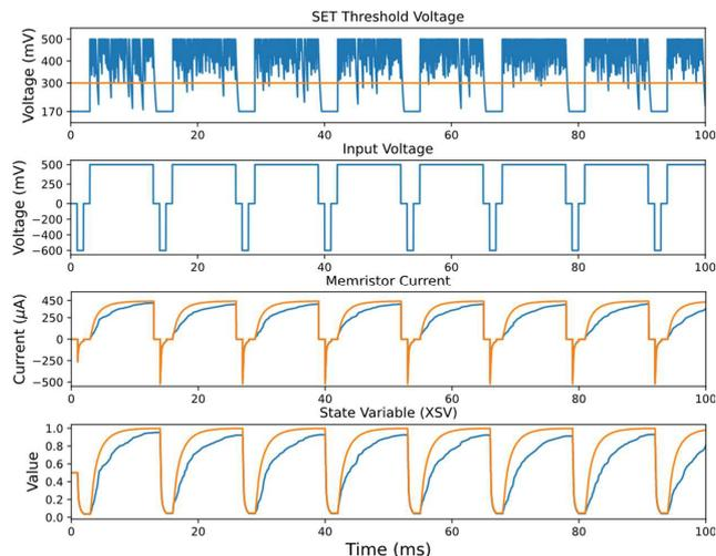
Fig. 6 Simulation results for the SET-RESET process based on the ReRAM model of [15]. From top to bottom, the plots include the situation with (blue) and without (orange) variability, distinguished with different color. They show the SET threshold value, the applied input voltage, the current through the memristor and the value of the state variable of the model, ranging between 0 and 1. SET threshold value was set to 0.3V when no variability was concerned.
