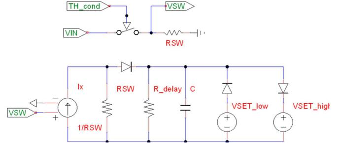
Fig. 3 Circuit implementing the variability of threshold value  $V_{SET}$ .
