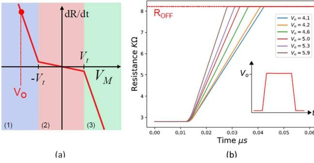
Fig. 1 (a) Graph indicating the dependence of the ReRAM device switching rate on the applied voltage  $V_M$ . (b)  $R$ - $t$  curves showing state evolution towards the HRS ( $R_{OFF}$ ) boundary by applying voltage pulses of different amplitude  $V_o$ . Model parameter values [5]:  $R_{ON} = 2800\Omega$ ,  $R_{OFF} = 8200\Omega$ , SET/RESET threshold  $v_t = 2.2V$ ,  $\alpha = 0$  and  $\beta = 1e11$ .
