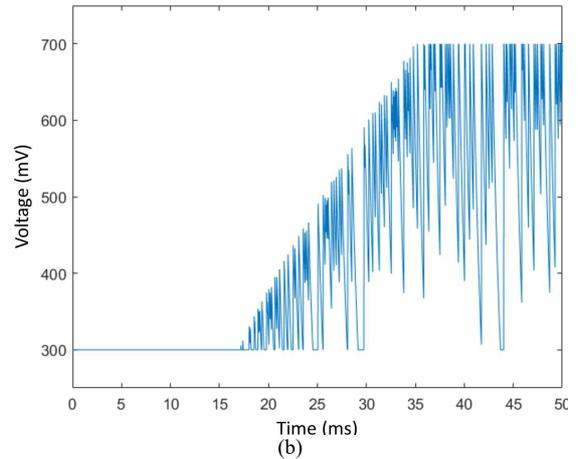
Fig. 5 Simulation results for the SET process based on the ReRAM model of [5]. (a) From top to bottom, the plots show the applied ramp voltage, the current through the device and its resistance, either with (orange) or without (blue) variability, distinguished with different line colors. (b) The time evolution of the value of the SET threshold parameter of the model.
