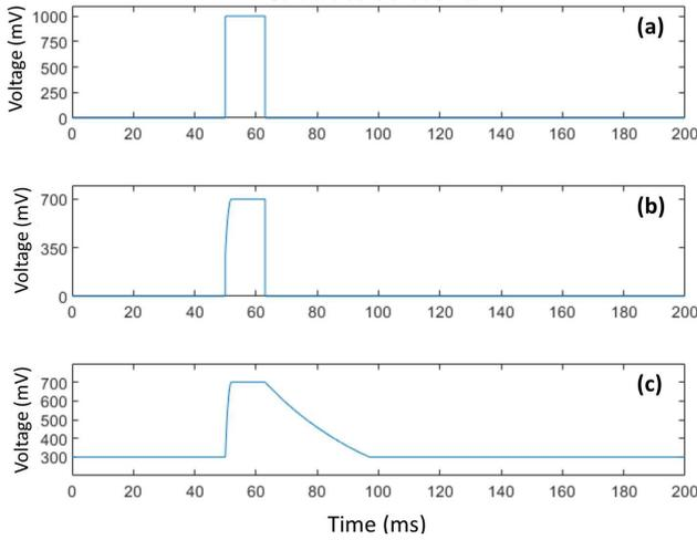
Fig. 4 Simulation results showing (a) the  $TH\_cond$  signal, (b) the  $VSW$  signal, and (c) the voltage across the capacitor.
