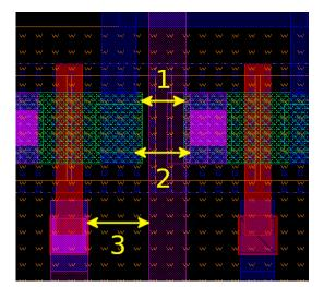
Fig. 4: (1) active-active spacing, (2) metal1-metal1 spacing, (3) metal2-metal2 spacing.
