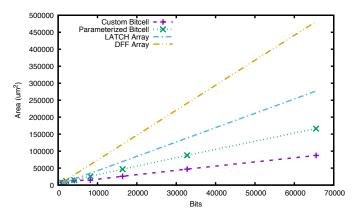
Fig. 9: FreePDK 45nm area comparison of 32-bit word memories of varying sizes shows both the custom and parameterized bitcell are more efficient than latch or DFF arrays.
