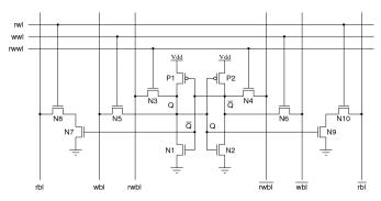
Fig. 3: A multi-ported SRAM cell has a single inverter pair (N1, P1, N2, P2) for storing a bit with a read/write port (N3, N4), write-only port (N5, N6), and read port (N7, N8, N9, N10) to share access to the differential storage nodes.
