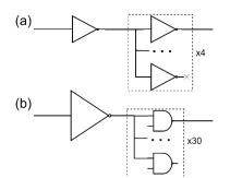
Fig. 6: Stage delays matched using similar size-fanout ratios with (a) using minimum sized inverters and dummy loads to match (b) the example wordline enable NAND fanout.
