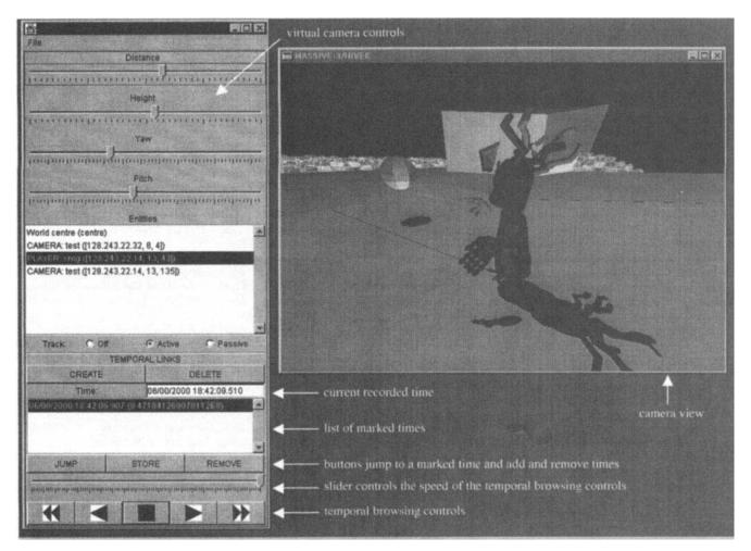
Figure 7. Graphical interface to the post-production
