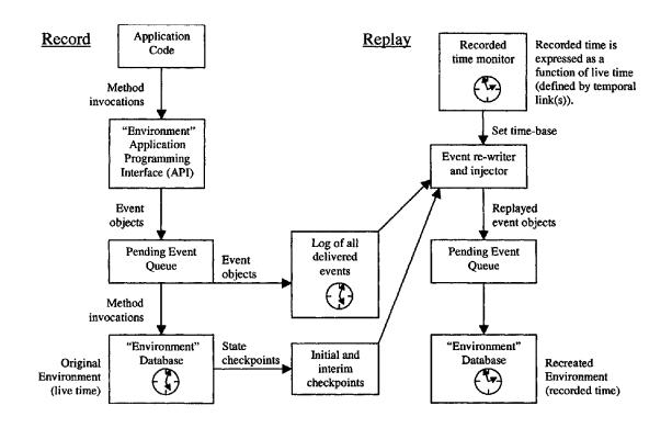
Figure 3. Record and replay in MASSIVE-3
