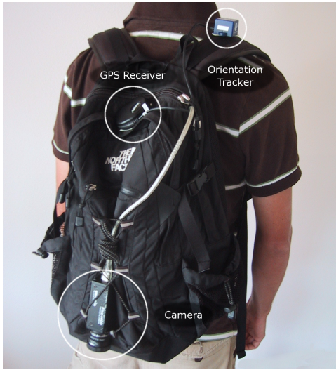
Figure 4: A wearable computer setup for GroundCam tracking. We use a Unibrain Fire-i 400 camera, an InterSense InertiaCube2 orientation tracker, and a Garmin GPS 18 receiver. Inside the backpack is a Dell Precision M50 laptop.
