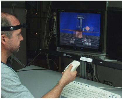
Figure 3: A user interacts with Dynallax, wearing a tracking sensor on a headband. Eventually, tracking will be camera-based and tetherless, as in other systems at EVL.
