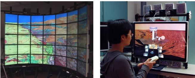
Figure 2: The Varrier AS VR system is shown in large tiled (left) and smaller desktop (right) versions.
