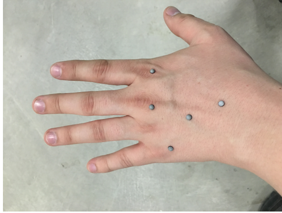
Figure 3.2: Example asymmetrical configuration of five 4mm markers on the hands. Used to create rigid bodies in Vicon Tracker for position and orientation tracking.
