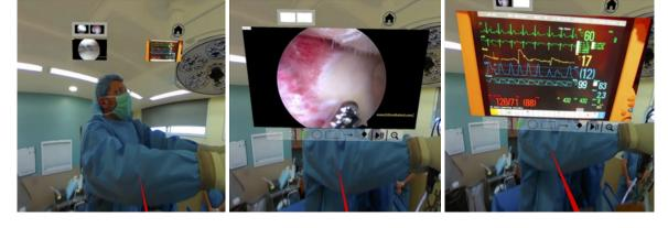
Figure 1: The SURVIVRS remote surgery guidance tool. (left) Immersive visualization of the surgery room offers a telepresence experience to the remote surgeon. (center) The local site of the surgery can be visualized in detail, where annotations can be sent to the surgery room. (right) Similarly, a live view of the patient vitals monitor is detailed to which the surgeon can make annotations.
