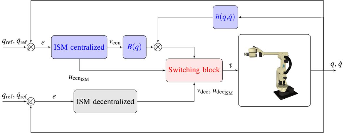
Fig. 1. The proposed multi-loop switching ISM control scheme
