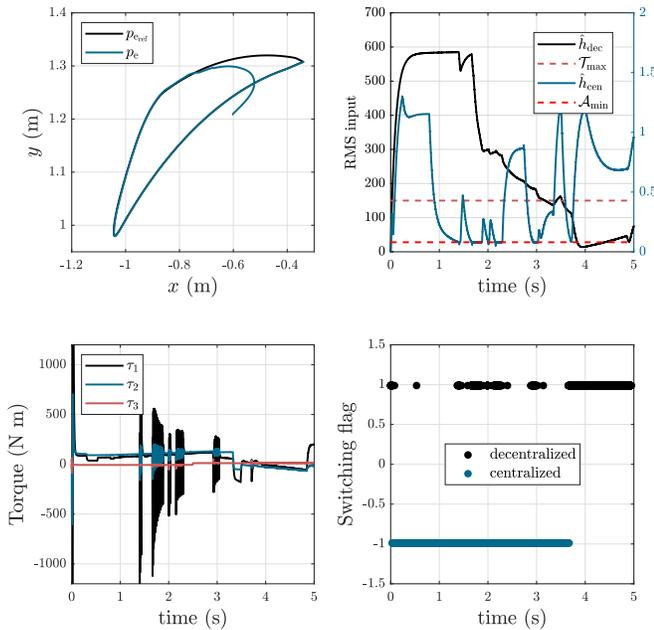
Fig. 2. From the top-left. Trajectory tracking in the operative space. RMS input of the switching block  $\hat{h}_{dec}$  (left-axis, black line),  $\hat{h}_{cen}$  (right-axis, blue line) and switching thresholds ( $\mathcal{T}_{max}$  in dashed dark-red line,  $\mathcal{A}_{min}$  in dashed light-red line). Control torques  $\tau$  for each joint. Switching flag, equal to 1 and -1 when Mode 1 (decentralized loop) or Mode 2 (centralized loop) is active
