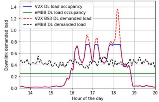
Fig. 10: Load occupancy for each slice in BS3 over time if 75% of resources are allocated to eMBB and 25% to V2X communications.
