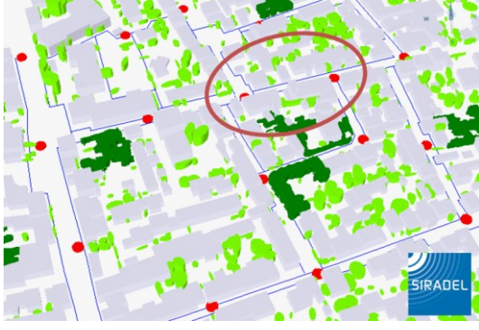
Fig. 5. Small-cell deployment (red dots) and user locations (sidewalks: blue lines) in real European city environment. The small-cells considered in this study are encircled.
