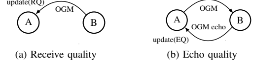
Fig. 4. B.A.T.M.A.N. local transmit quality estimation from B-A utilizing receive and echo quality estimated both from the last N received OGM messages.
