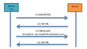
Figure 1. SIP extension: Device UA registration with its device description
