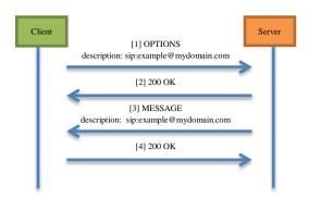
Figure 3. SIP extension: complete device description retrieval
