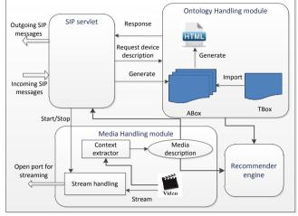
Figure 5. SIP Server-side application architecture
