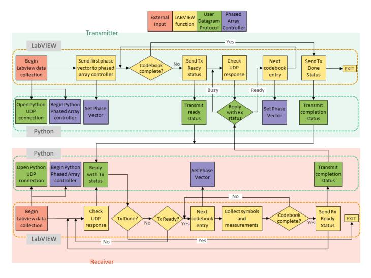
Fig. 2. Figure representing the proposed prototype's flow of control between the receiver and transceiver during training via user-defined Python and LabVIEW interfaces.
