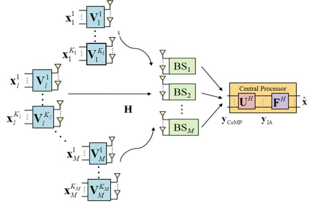
Fig. 1. Illustration of centralized IA aided UL CoMP system model.
