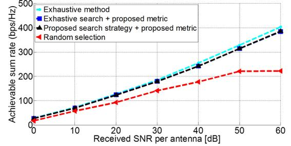
Fig. 3. The achievable sum rates of various configuration selection schemes with  $\epsilon = 0.4$ ,  $N_t = 8$ ,  $N_r = 8$ ,  $K = 3$ , and  $M = 3$ .
