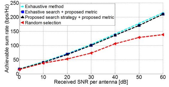
Fig. 4. The achievable sum rates of various configuration selection schemes with  $\varepsilon=0.9$ ,  $N_t=4$ ,  $N_r=4$ ,  $K=3$ , and  $M=3$ .
