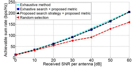
Fig. 2. The achievable sum rates of various configuration selection schemes with  $\epsilon = 0.4$ ,  $N_t = 4$ ,  $N_r = 4$ ,  $K = 3$ , and  $M = 3$ .
