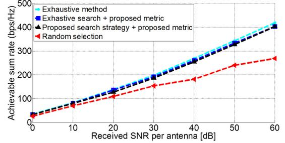
Fig. 5. The achievable sum rates of various configuration selection schemes with  $\varepsilon=0.9$ ,  $N_t=8$ ,  $N_r=8$ ,  $K=3$ , and  $M=3$ .
