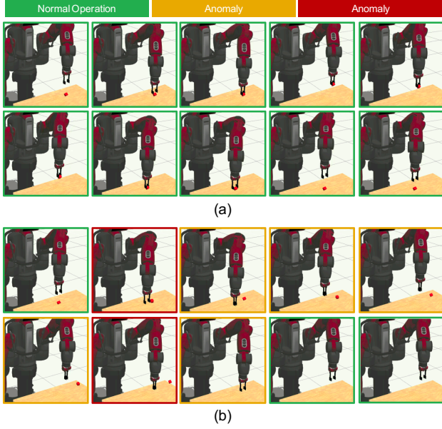
Figure 5. Robot surveillance video sequence (we show only 1 frame in 1 second). Outline color of each frames shows if the systems recognized it as an anomaly or not. (a) Normal pick and place operation with no anomaly. (b) Failed operation results in the ball rolling off the table.
