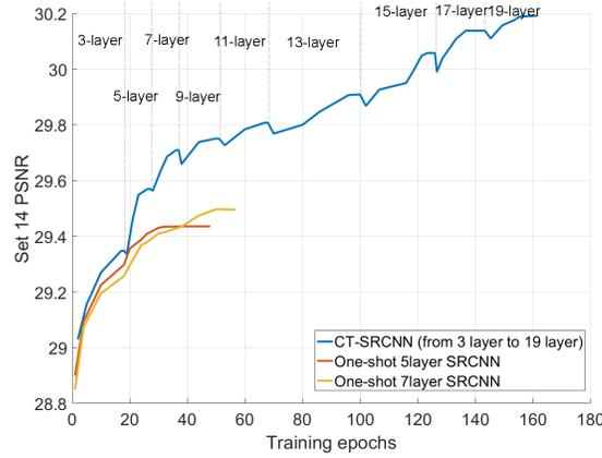
Figure 7. Epochs vs. Set14 PSNR of CT-SRCNN and one-shot trained SRCNNs.
