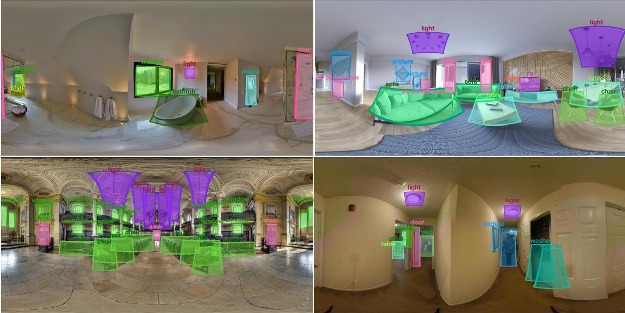
Figure 1: Examples of the images overlaid with labeled Bounding Field-of-VIEWS (BFoVs) as well as object categories (text and color-code) in our 360-Indoor dataset.
