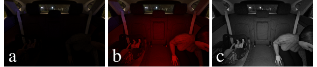
Figure 6. Comparison between a standard RGB image and our simple approach to imitate an active infrared camera system for a dark scenery. a) Standard RGB image in environmental lighting. b) RGB image of the scenery illuminated by an active red light. c) Red channel only of the RGB image of the illuminated scenery (used as infrared imitation in SVIRO).
