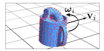
Figure 2. Problem input. Our method uses a point cloud (red spheres) and initial linear  $\mathbf{v}_i$  (arrow) and angular velocity  $\boldsymbol{\omega}_i$  (circular arrow) to predict dynamics. The object is assumed to move on a plane but can exhibit wobbling or complete toppling.
