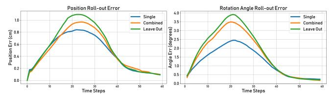
Figure 4. Roll-out errors for object generalization experiments. Each curve shows the median roll-out error over all evaluation datasets using that training procedure. Separate models trained on each dataset are shown by the blue curves, a single model trained on the Combined dataset then evaluated on individual datasets is shown by the orange curve, and separate models trained on the Combined dataset with the evaluation shape category left out are shown in green.
