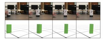
Figure 6. Real-world data. We captured 66 sequences of a box with a motion capture system and trained our method on the captured data. The top row shows an external view of one of the test trials. The bottom row shows predictions.
