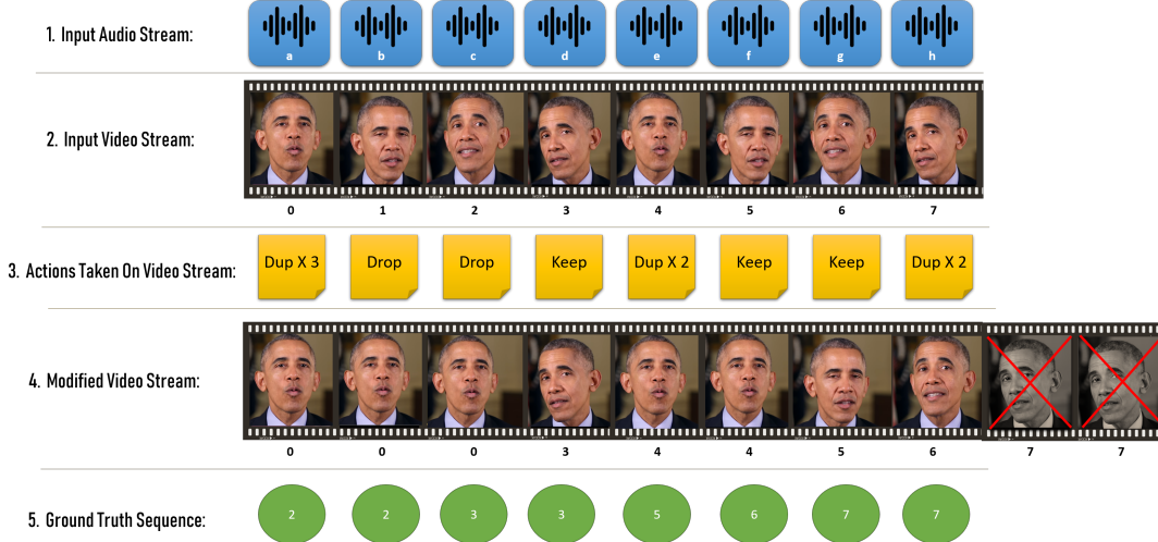
Figure 3: The creation process of a training audio-video pair, along with its ground truth labels. For a given audio-video pair (1, 2), a sequence of random actions is taken (3) on the visual stream, to create an unsynchronized video stream (4) along with the ground truth labels (5). The resulted training pair consists of the input audio (1) and the modified video stream (4) and the task is to predict the ground truth labels (5). Note that the frames at the end of the modified video stream are removed since they fall after the audio boundaries.
