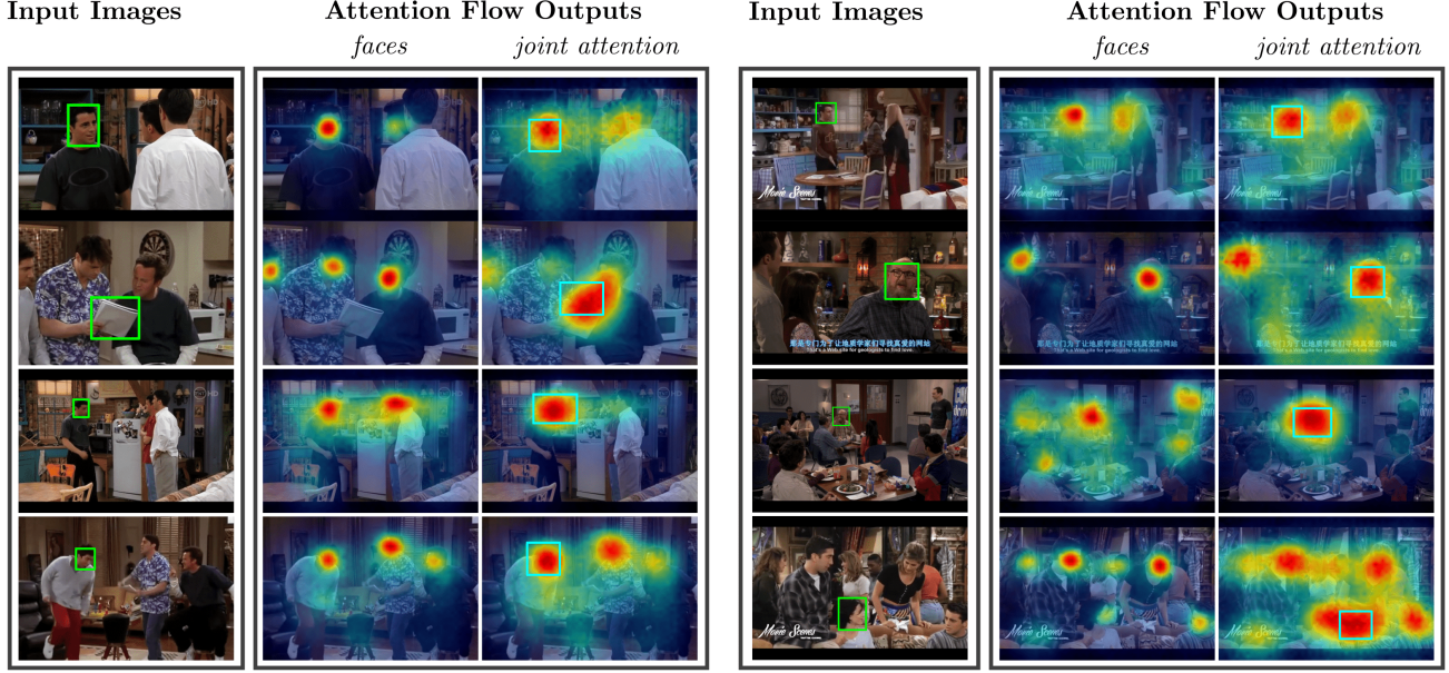
Figure 5. Qualitative results of Attention Flow Bounding boxes on sample test images (green) show the ground truth attentional focus. The second and third columns are our estimated Attention Flow. In the third column, we also depicted the estimated bounding boxes (cyan). Figure best viewed in color.
