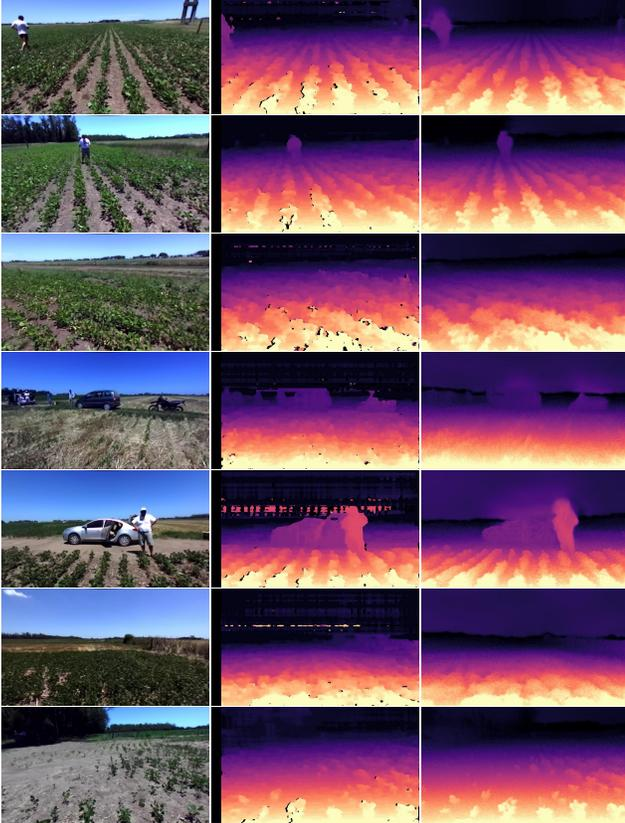
Figure 4. **Qualitative results of self-supervised monocular depth estimation on Rosario [45].** First column: selected raw RGB images; Second column: ground truth depth images generated with SGBM [31]; Third column: predicted depth using Monodepth2 [26] with mixed training strategy (MS\*). More results please see supplementary material.
