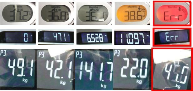
date, for other meters one tag is sufficient. For the glucose meter 556 screen snapshots were recorded, and for all other meters 50 images per device were collected. Dataset details can be found in Table 2.
