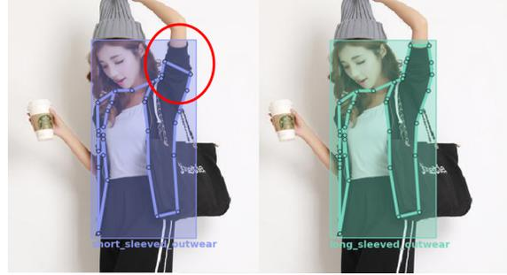
Figure 5. Detection results for two different classes. The keypoint score for the right class has a higher value. Short sleeved outerwear on the left has  $Score_{bbox} = 0.31$ ,  $Score_{kps} = 0.28$ . Long sleeved outerwear on the right has  $Score_{bbox} = 0.29$ ,  $Score_{kps} = 0.36$ .
