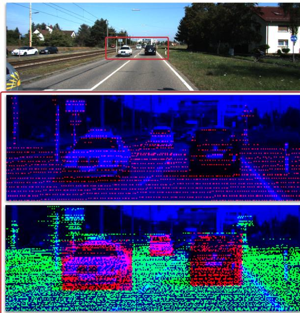
Figure 1. **Top:** an input image, **middle:** a cropped, zoomed-in image, where **red** points represent LiDAR returns projected onto the image plane, **bottom:** multi-scale dense voxel centers projected onto the image plane, where **green** and **red** points are associated with background and foreground voxel features, respectively. DVF increases the number of correspondences between image and LiDAR features.
