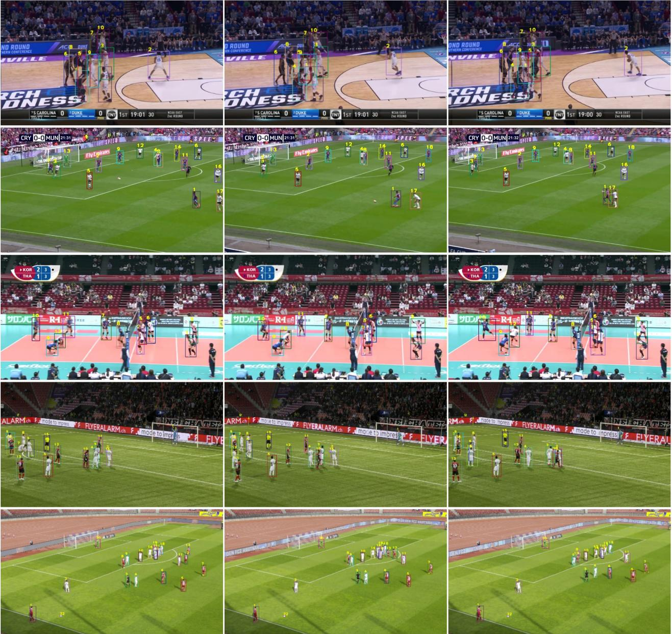
Figure 6. Visualization results of Deep-EIoU from random sampled clips of SportsMOT dataset (row 1 to 3) and SoccerNet-Tracking dataset (row 4 to 5). With the iterative scale-up ExpansionIoU and deep features association, our algorithm can achieve robust multi-athlete tracking under severe occlusion conditions in multiple diverse sports scenarios including basketball, football, and volleyball. More visualization results can be found in supplementary material.
