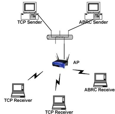
Figure 1. Network setup for ABRC scheme
