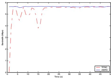
**Figure 2. Dynamic bandwidth usage of TFRC and ABRC when there is no other competing traffic**
