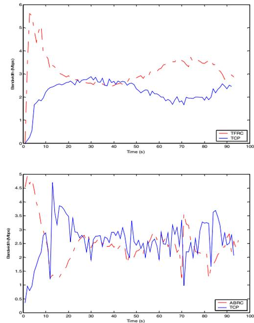
**Figure 3. Dynamic bandwidth usage of TFRC /ABRC versus bandwidth usage of competing TCP traffic**
