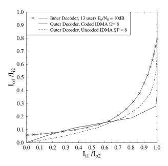
Fig. 3. EXIT chart analysis of coded IDMA over AWGN channels for a bandwidth expansion of  $\Omega=8,\,13$  users and  $E_b/N_0$  = 10dB.
