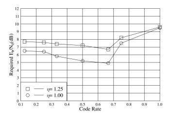
Fig. 6. The  $E_b/N_0$  values required for supporting a normalised user-load of  $\eta$  versus the code-rate at a fixed bandwidth expansion factor of  $\Omega = 8$  and for  $P_e = 10^{-5}$  using the convolutional codes of Table I
