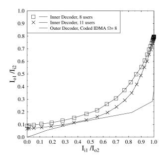
Fig. 4. EXIT charts for different number of users supported in coded IDMA over AWGN channels at a bandwidth expansion factor of  $\Omega = 8$  and  $E_b/N_0 = 10$ dB, using R = 1/2 convolutional coding
