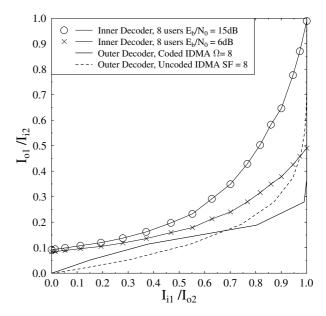
Fig. 2. EXIT chart analysis of coded IDMA over AWGN channels for a bandwidth expansion of  $\Omega = 8$ , K = 8 users and various  $E_b/N_0$  values.
