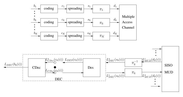
Fig. 1. Transmitter of single-carrier IDMA and its joint soft-in-soft-out multiuser detector, de-spreader (Des) and channel decoder (CDec)
