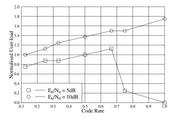
Fig. 5. Normalised user-load versus code-rate for a fixed bandwidth expansion factor of  $\Omega = 8$  and for  $P_e = 10^{-5}$  using the convolutional codes of Table I
