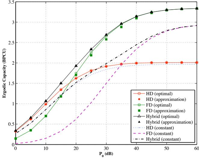
Fig. 3. Ergodic capacity versus  $P_0$  for optimal and approximated time split;  $\omega_{\text{HD}}^* = 1/3$  and  $\omega_{\text{FD}}^* = 1/2$  for constant time split,  $\sigma_{S,R}^2 = \sigma_{R,D}^2 = \sigma_{R,R}^2 = 1$ ,  $\omega_0 = 0.1$ ,  $\delta = 20$  dB.
