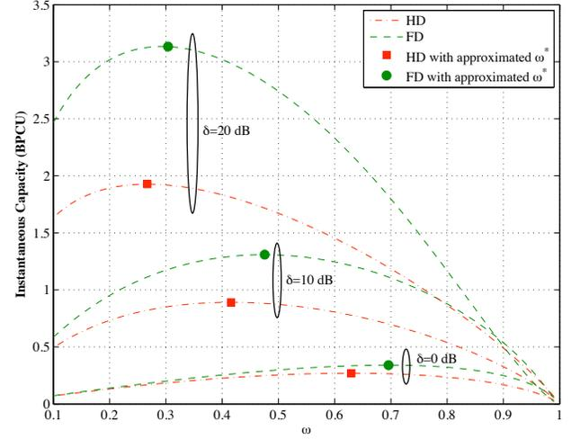
Fig. 5. Instantaneous capacity versus  $\omega$ ;  $f = 2.83$ ,  $g = 0.5122$ ,  $h = 0.91$ ,  $\delta = \{0, 10, 20\}$  dB,  $P_0 = 40$  dB and  $\omega_0 = 0.1$ .
