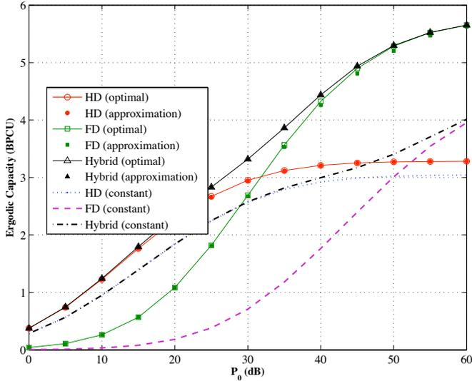
Fig. 4. Ergodic capacity versus  $P_0$  for optimal and approximated time split;  $\omega_{\text{HD}}^* = 1/3$  and  $\omega_{\text{FD}}^* = 1/2$  for constant time split,  $\sigma_{S,R}^2 = \sigma_{R,D}^2 = \sigma_{R,R}^2 = 1$ ,  $\delta = 30$  dB and  $\omega_0 = 0.1$ .
