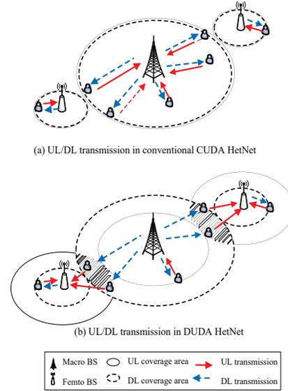
Fig. 1. Illustration of UL and DL coverage for a two-tier HetNet in DUDA and CUDA scenarios respectively.
