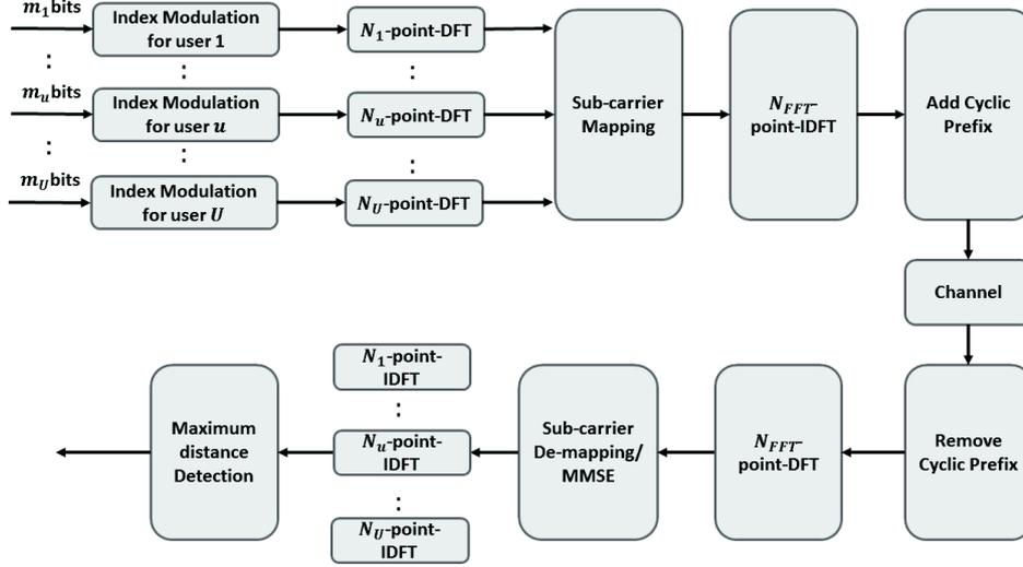
Figure 1: SC-FDMA-IM transceiver.
