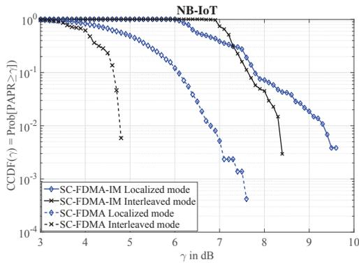
Figure 4: PAPR performance for SC-FDMA-IM in NB-IoT scenario.
