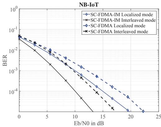
Figure 6: BER performance for SC-FDMA-IM in NB-IoT scenario.
