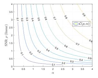
Fig. 3. Contour plot of  $C(\rho, \alpha)$  (4) with  $\alpha \leq 4$  and  $\rho \leq 4$ . The gap between the adjacent contours becomes large as  $C(\rho, \alpha)$  increases, which shows the increasing demands on  $\rho$  and  $\alpha$  to increase  $C(\rho, \alpha)$ .
