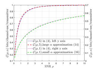
Fig. 5. The comparison between the capacity  $C(\rho, \alpha)$  (4) with large  $\alpha$  ( $\alpha = 5$ ), small  $\alpha$  ( $\alpha = 1$ ) and their corresponding approximations in (14) and (16). The good approximations over a wide range of SNR shows that  $\alpha = 5$  is big enough and  $\alpha = 1$  is small enough to use (14) and (16) for accurate approximations.
