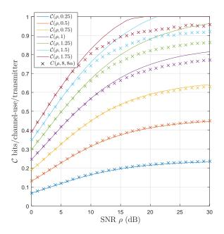
Fig. 1. Comparison between  $C(\rho, M, \alpha M)$  (2) and  $C(\rho, \alpha)$  (4) with M = 8 for  $\alpha \in \{0.25, \dots, 1.75\}$  with SNR varying from 0 dB to 30 dB. The accuracy of the approximation in a wide range of SNR shows that M = 8 is big enough to get a valid approximation with  $C(\rho, \alpha) \leq 0.7$ .
