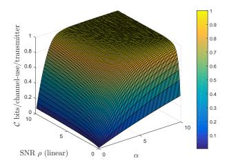
Fig. 2.  $C(\rho, \alpha)$  (4) versus  $\rho$  and  $\alpha$  with  $0.1 \le \rho \le 10$  and  $0.1 \le \alpha \le 10$ .  $C(\rho, \alpha)$  increases linearly with  $\rho$  and  $\alpha$  when  $\rho$  and  $\alpha$  are small but  $C(\rho, \alpha)$  "saturates" quickly.
