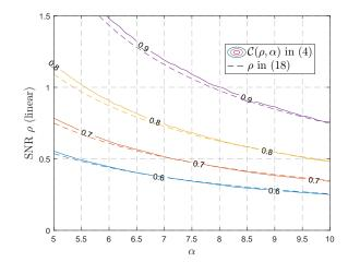
Fig. 6. Comparison between the actual SNR  $\rho$  and the approximated SNR (18) for the contours  $C = 0.6, \ldots, 0.9$ . The solid lines are contour plots of (4), and the dashed lines present the approximation of  $\rho$  (18) as a function of  $\alpha$ .
