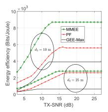
Figure 3: The weakest user's performance with different designs at different weak users' distances from the BS.
