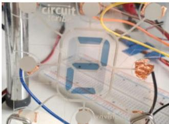
Fig.10. Electrochromic seven segment display developed by Ynvisible.
