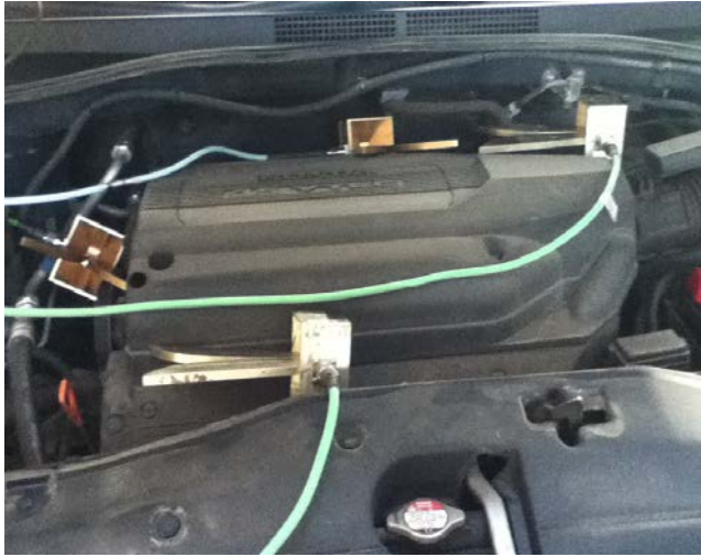
Figure 4. Channel measurement in the engine compartment
