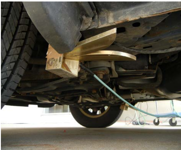
Figure 3. Channel measurement beneath the chassis
