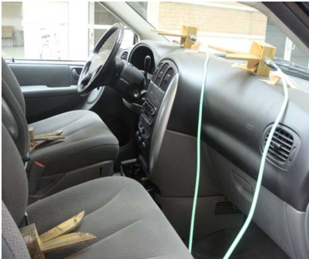
Figure 2. Channel measurement in the car compartment
