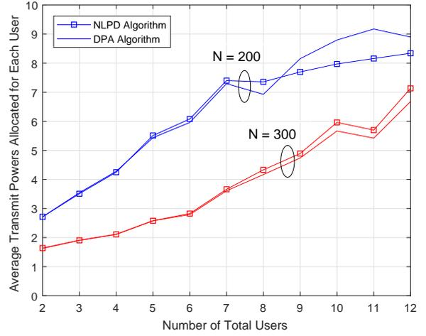
Fig. 2: Average transmit powers allocated for each user versus the number of total users.
