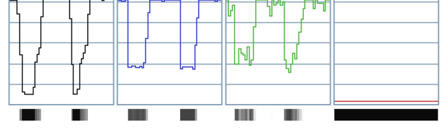
Figure 7. Example sensor output, with bars indicating the sensed data as the robot sweeps over a black line. Left to right: ideal sensor, ambient light added, A/D noise added, sensor value stuck.
