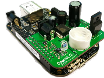
Fig. 1: OpenVLC1.3 cape on top of an embedded board.
